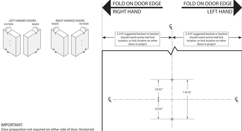
center line from finish floor is 36" or as desired. Mark 2 holes then install mounting screws on black marks.
